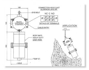
The switch is hung from L/S stock pipe top. The height depends on the position at which action is desired. To enable tilting of the switch 30 cm long GI conduit pipe is fixed on the switch, so that when the tip of the conduit pipe touches the material the switch tilts. This causes change in status i.e. Contacts changeover
