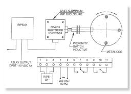
Pairs of magnet are attached to the shaft or coupling to be monitored so that they rotate past a magnetic switch (pulse generator) and they operate the magnetic switch with their magnetic fields, without contact and without wear and tear. The magnetic switches used have a practically unlimited service life and are connected to a motion
