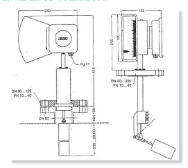
Revathi-Helios Level Transmitters are having 2 systems i.e. The immersed body displacer and high grade instrument combination with electronic angle transmitter. The rotation of the extended pointer shafts picked up contactless by a capacitive bridge amplified and converted with an impressed standard signal. In combination with a intrinsically safe power pack the transmitter satisfies the explosion safety regulation may be employed in the rooms where there is an explosion hazard.
