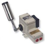
edge to allow normally accepted swaying. When the swaying exceeds allowable limit, the belt edge would push the contact roller which in turn would actuate the switch. When swaying stops the switch would automatically reset under the action of resetting spring.
